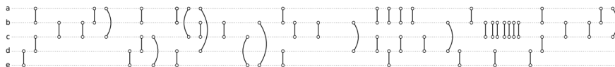
Figure 1: A link stream. The x-axis represents time, while the y-axis represents nodes. Edges arrive between nodes over time.
